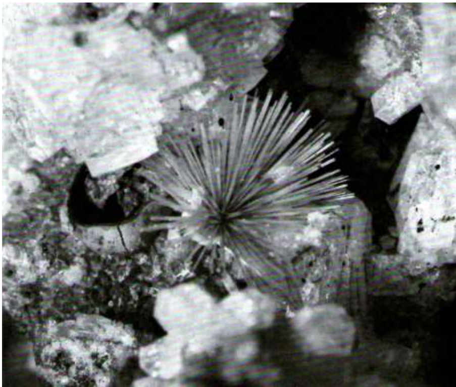
Fig. 2. Bundle of mazzite needles associated with white rhombohedra of chabazite and white pseudotetragonal phillipsite twins (field of view approx. 1x1 cm). From Galli et al., 1974.
